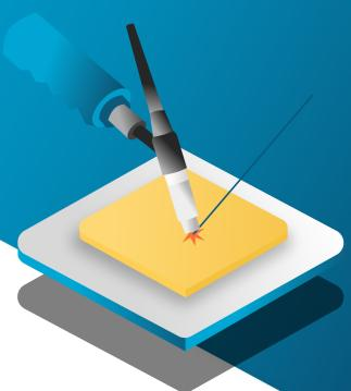
TIG (Tungsten Inert Gas) welding is a precision welding process that uses a non-consumable tungsten electrode to produce the weld. An inert gas, usually argon or helium, shields the weld area from atmospheric contamination.
